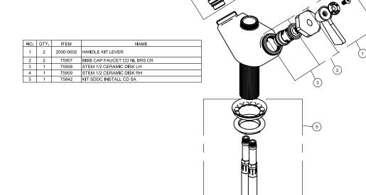
PRODUCT SPECIFICATIONS: SINGLE DECK DUAL CONTROL MOUNT MIXING FAUCET, QUARTER TURN CERAMIC DISC CARTRIDGES WITH LEVER HANDLES, 1/2" FEMALE NPT INLET. PRODUCT COMPLIANCE: ASME A112.18.1 / CSA B125.1 NSF 61 - Section 9 NSF 372 (Low Lead Content)
