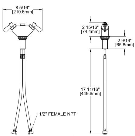
PRODUCT SPECIFICATIONS: SINGLE DECK DUAL CONTROL MOUNT MIXING FAUCET, QUARTER TURN CERAMIC DISC CARTRIDGES WITH LEVER HANDLES, 1/2" FEMALE NPT INLET. PRODUCT COMPLIANCE: ASME A112.18.1 / CSA B125.1 NSF 61 - Section 9 NSF 372 (Low Lead Content)
