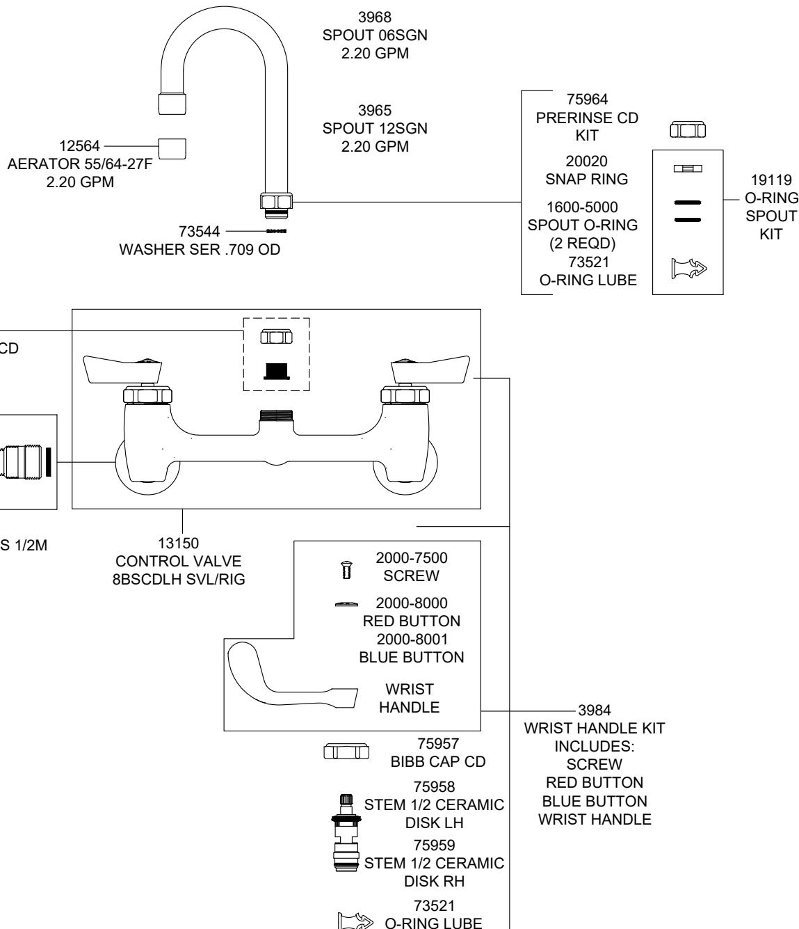
PRODUCT SPECIFICATIONS: 8" BACKSPLASH FAUCET, QUARTER TURN CERAMIC DISK CARTRIDGES W/ CHECK STEMS, WRIST HANDLES, 6" OR 12" SWIVEL OR RIGID GOOSENECK SPOUT W/ 2.2 GPM @ 60 PSI AERATOR, 1/2" NPT MALE INLETS W/ CLOSE ELBOW 1/2" NPT FEMALE INLETS
