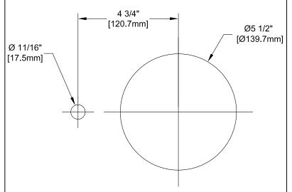
NOTE: THIS ONLY APPLIES TO FISHER 'S DIPPERWELL. IF FAUCET IS INSTALLED TO CLOSE WILL NOT BE ABLE TO REMOVE PAN OR IF FAUCET INSTALLED TOO FAR WATER WILL SPILL ON COUNTER.
